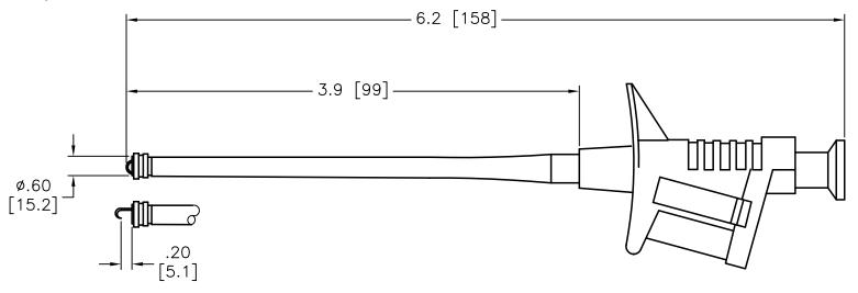
Hook style contact can fit terminals up to .20 [5mm] and can be rotated for easy connection. Flexible shaft is bendable to  $\pm 90^{\circ}$ .
