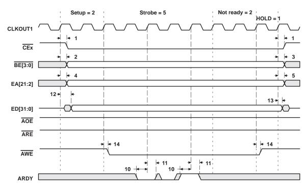
Figure 14. Asynchronous Memory Write Timing
