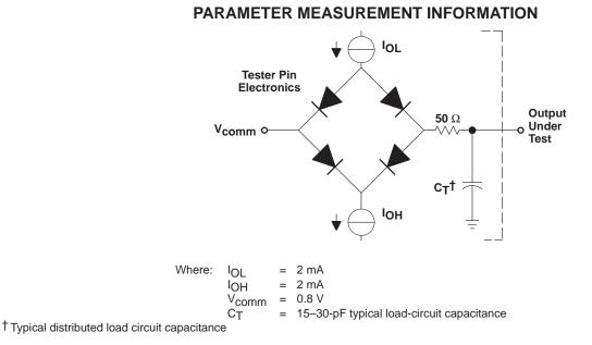
Figure 6. TTL-Level Outputs
