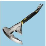
A multi-purpose four in one tool for prying, splitting, board bending, and striking jobs. A one piece forged construction for increased durability with textured grip for comfort and control even when wet. Features bevelled nail slot for pulling and prying along with two tiered jaws for common dimensional timber and decking.
