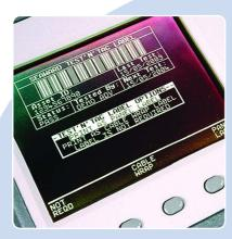
2. On completion of the test routine, choose between panel label and cable wrap label
