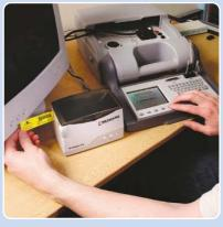
3. Label is printed automatically from the tester
