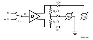
FIGURE 1. Differential Driver DC Test Circuit
