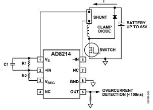
Figure 31. High Side Overcurrent Protection
