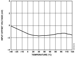
Figure 6. Input Offset Voltage vs. Temperature
