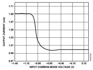
Figure 5. Output Current (Output High) vs. Input Common-Mode Voltage (With Respect to V<sub>s</sub>)
