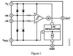
voltages are referenced to the supply voltage, as is the internal 2.4 V regulator. The input-to-output response time is typically <100 ns.
