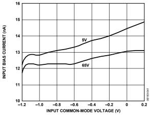
Figure 4. Input Bias Current vs. Input Common-Mode Voltage (With Respect to V<sub>5</sub>)
