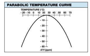
To determine frequency stability, use parabolic curvature (k). For example: What is stability at 45 °C?
