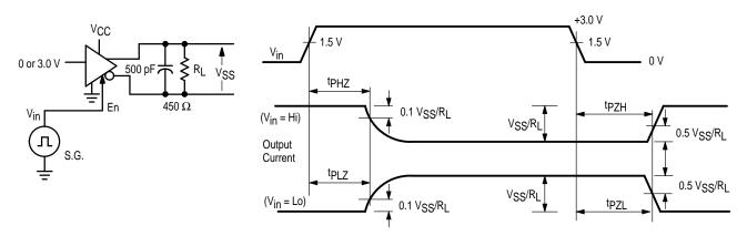
**NOTES:** 1. S.G. set to:  $f \le 1.0$  MHz; duty cycle = 50%;  $t_p$ ,  $t_f$ ,  $\le 10$  ns. 2. Above tests conducted by monitoring output current levels.
