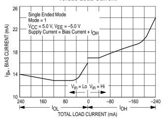
Figure 13. Internal Negative Bias Current versus Load Current
