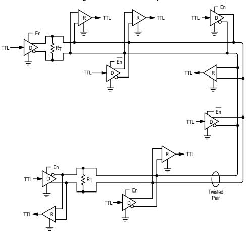
NOTES: 1. Terminating resistors R<sub>T</sub> should be located at the physical ends of the cable.
