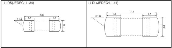
\*Copper plate area dimensions above are reference dimensions with being soldered with conditions bellow.
