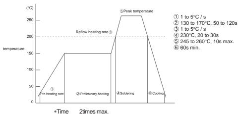
Recommended peak temperature is over 245°C. If peak temperature is below 245°C, you may adjust the following parameters; Time length of peak temperature (longer), Time length of soldering (longer), Thickness of solder paste (thicker).
