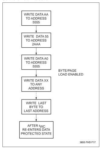
Regardless of whether the device has previously been protected or not, once the software data protection algorithm is used and data has been written, the X28C256 will automatically disable further writes unless another command is issued to cancel it. If no further commands are issued the X28C256 will be write protected during power-down and after any subsequent power-up.
