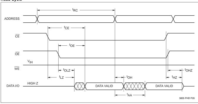
Note: (5)  $t_{LZ}$  min.,  $t_{HZ}$ ,  $t_{OLZ}$  min., and  $t_{OHZ}$  are peridocally sampled and not 100% tested.  $t_{HZ}$  and  $t_{OHZ}$  are measured, with  $C_L$  = 5pF, from the point when  $\overline{CE}$  or  $\overline{OE}$  return HIGH (whichever occurs first) to the time when the outputs are no longer driven.
