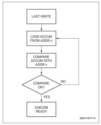
The Toggle Bit can eliminate the software housekeeping chore of saving and fetching the last address and data written to a device in order to implement  $\overline{\text{DATA}}$  Polling. This can be especially helpful in an array comprised of multiple X28C256 memories that is frequently updated. The timing diagram in Figure 4 illustrates the sequence of events on the bus. The software flow diagram in Figure 5 illustrates a method for polling the Toggle Bit.
