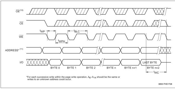
Notes: (10) Between successive byte writes within a page write operation,  $\overline{\text{OE}}$  can be strobed LOW: e.g. this can be done with  $\overline{\text{CE}}$  and  $\overline{\text{WE}}$  HIGH to fetch data from another memory device within the system for the next write; or with  $\overline{\text{WE}}$  HIGH and  $\overline{\text{CE}}$  LOW effectively performing a polling operation.
