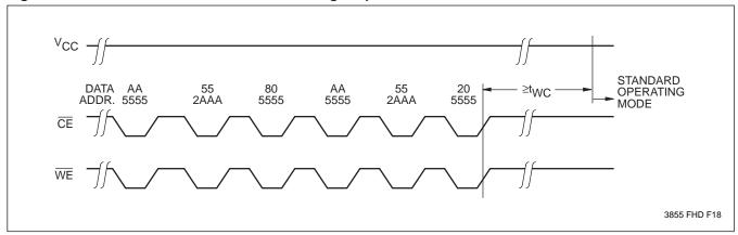
Figure 9. Software Sequence to Deactivate Software Data Protection
