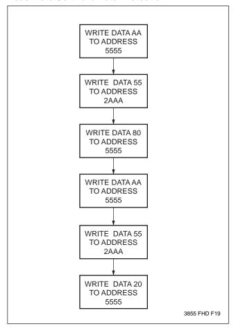
In the event the user wants to deactivate the software data protection feature for testing or reprogramming in an E<sup>2</sup>PROM programmer, the following six step algorithm will reset the internal protection circuit. After  $t_{WC}$ , the X28C256 will be in standard operating mode.
