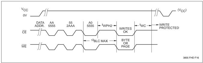
Figure 7. Write Sequence for Software Data Protection
