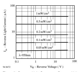
Figure 5. Reverse Light Current vs. Reverse Voltage
