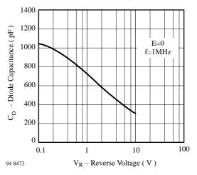
Figure 6. Diode Capacitance vs. Reverse Voltage
