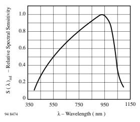
Figure 7. Relative Spectral Sensitivity vs. Wavelength
