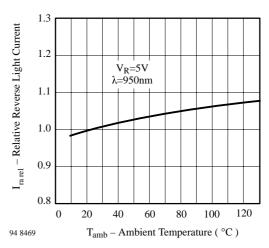
Figure 2. Relative Reverse Light Current vs.
