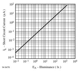
Figure 3. Short Circuit Current vs. Illuminance
