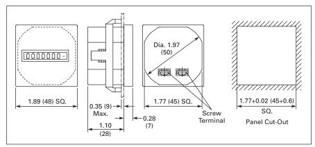
Figure 59. 1/16th DIN Hour Meters — Approximate Dimensions in Inches (mm)
