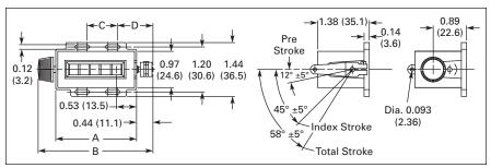
Figure 1. X Series — Approximate Dimensions in Inches (mm)
