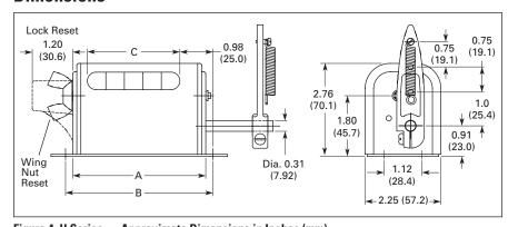
Figure 4. H Series — Approximate Dimensions in Inches (mm)
