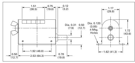
Figure 16. D-7 Series — Approximate Dimensions in Inches (mm)
