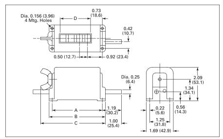
Figure 13. CS Series — Approximate Dimensions in Inches (mm)
