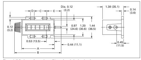
Figure 8. X Series — Approximate Dimensions in Inches (mm)
