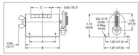
Figure 5. D Series — Approximate Dimensions in Inches (mm)
