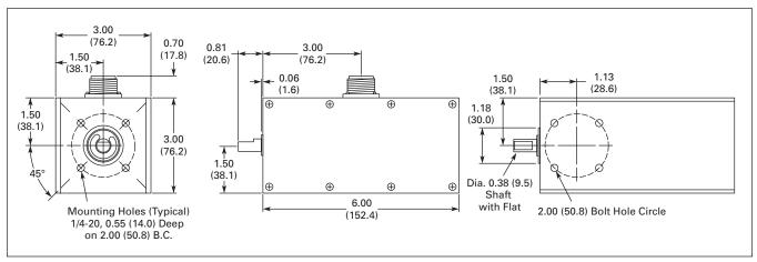
Figure 72. Heavy Duty Encoder — Approximate Dimensions in Inches (mm)
