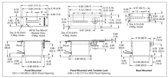
Figure 35. MF Series — Approximate Dimensions in Inches (mm)
