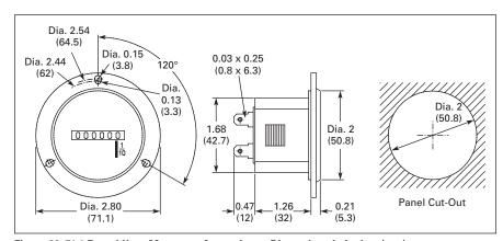
Figure 60. 71.1 Round Hour Meters — Approximate Dimensions in Inches (mm)
