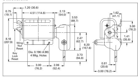
Figure 32. HF Series — Approximate Dimensions in Inches (mm)
