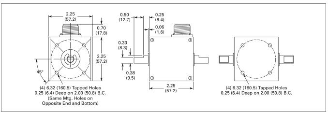
Figure 71. Cube Shaft Encoders — Approximate Dimensions in Inches (mm)
