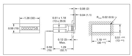
Figure 33. Micro Display Counter — Approximate Dimensions in Inches (mm)
