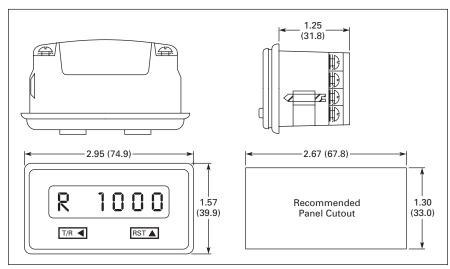
Figure 39. Courier Series Totalizers — Approximate Dimensions in Inches (mm)
