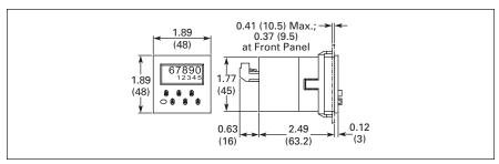
Figure 62. Battery-Powered LCD Time Control, 48 x 48 mm — Approximate Dimensions in Inches (mm)
