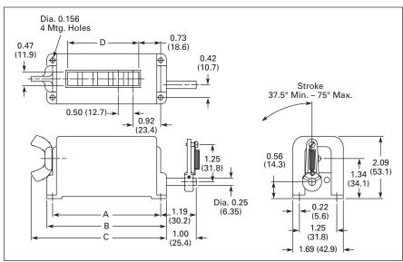
Figure 2. CS Series — Approximate Dimensions in Inches (mm)
