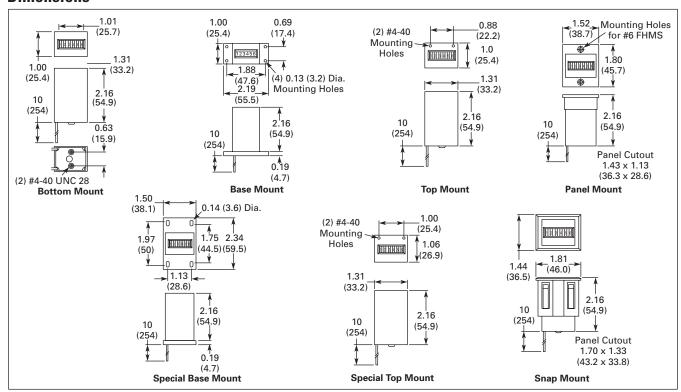
Figure 34. SE Series — Approximate Dimensions in Inches (mm)
