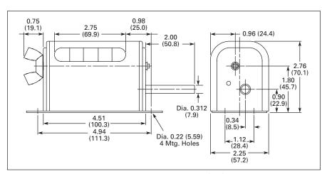
Figure 22. HDW Series — Approximate Dimensions in Inches (mm)
