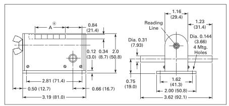
Figure 19. D-6 Series — Approximate Dimensions in Inches (mm)
