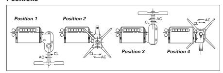
Figure 31. HF Series — Can Counter Positions
