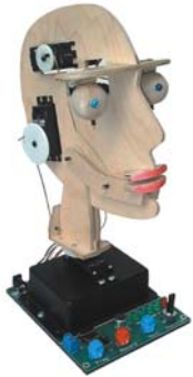
Alex animated head can be programmed using the development board and the actuators panel
