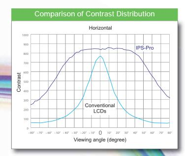
"IPS-Pro has a much higher and more stable image performance over viewing angle than any other TFT technology."
