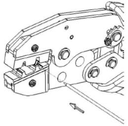
Then, insert the cable into the open barrel. After that, squeeze the handle at the till ratchet released.
