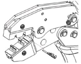
First, to place the open barrel into the die set.
