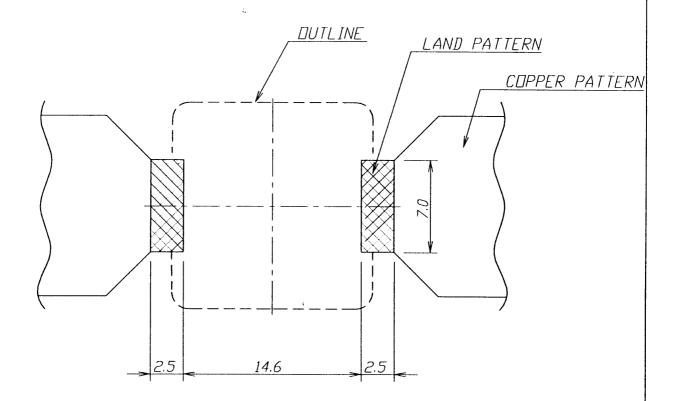
The customer shall determine the land dimensions shown above after confirming accessibility regarding mounting and safety.
