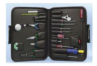
This tool kit contains all the tools an electronic engineer should need to carry out day to day contracts. The PU carrying case measures 400x295x70mm and is fitted with all the necessary attachments required to securely hold the tools.
