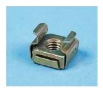
A range of zinc plated cage nuts available in M5 and M6 thread sizes. The nuts are held in a spring steel cage. Ideal for use when fixing front panels onto racking systems, cabinets etc Two types of cage nuts are available when using different thickness materials. Each pack contains 25 nuts.
