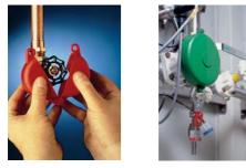
Ensures an effective safeguard against accidents involving gate valves. Made from durable polypropylene with stainless steel hinges for added strength and security, preventing tampering. Unlike lockouts without a steel hinge these lockouts cannot be popped open. The knockout centre enables these lockouts to take a rising gate valve.
