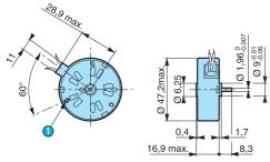
1 3 fixing holes ØM2 at 120 ° on r=19.5 max. depth 2.4 mm
