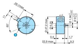
1 3 fixing holes Ø M2 at 120  $^{\circ}$  on r=19.5 max. depth 3.5 mm
