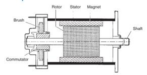
The stator is formed by a metal carcass and one or more magnets that create a permanent magnetic field inside the stator. At the rear of the stator are the brush mountings and the brush gear which provide electrical contact with the rotor.
