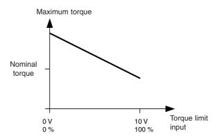
When the torque limit is reached, the motor does not follow its speed setpoint, but maintains a constant torque equal to this limit, as long as its speed remains below the setpoint.
