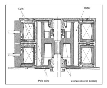
Synchronous motors with a single-phase AC voltage and a permanent magnet must have, for reverse operation, at least 2 stators and 2 coils. Reverse operation can be achieved electrically using a single-pole switch.
