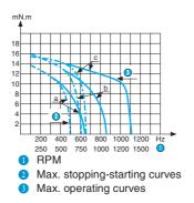
Max. stopping-starting frequency curves as a function of the external inertia load at zero antagonistic torque. Tests at constant U.
