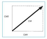
Cm = Holding torque of the motor energised «two phases at a time»
