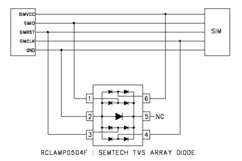
The single TVS diode or varistor can be used on the respective pins.
