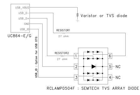
The single TVS diode or varistor can be used on the respective pins. Additionally Telit recommend that suitable resistors should be used to protect the USB D+/D- signal from ESD.
