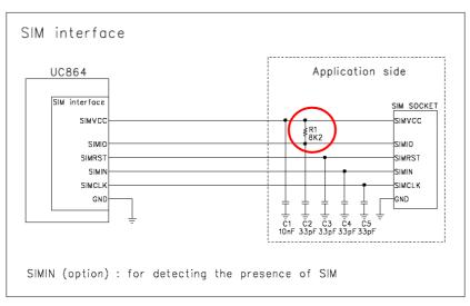
All the components in the application side (dotted line above) should be included into the application board and the recommended values should be referred as well.
