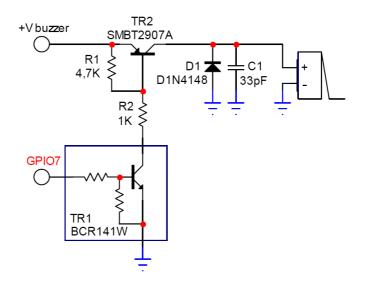
Example of Buzzer's driving circuit.
