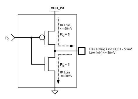
output PAD equivalent circuit
