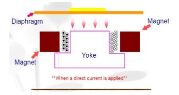
Drawing of the Magnetic Buzzer.
