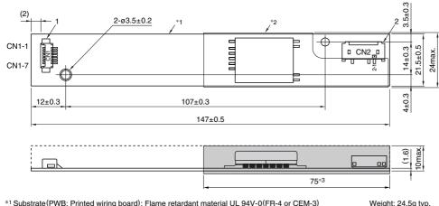
\*1 Substrate (PWB: Printed wiring board): Flame retardant material UL 94V-0(FR-4 or CEM-3)
