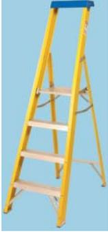
Manufactured from glass fibre channel stiles and fitted with serrated aluminium treads. The hinge operation is designed not to trap fingers. Fitted with slip resistant feet and tool holes. Conductivity tested to 30,000 volts and will meet all the latest electrical standards. Certified to EN131.
