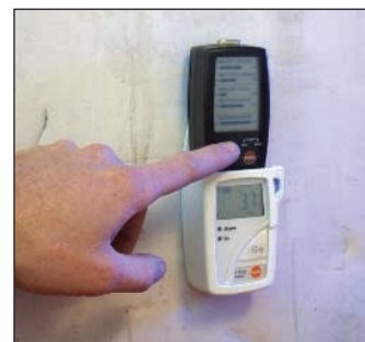
Collects data on-site, downloads and analyses centrally on PC. The high-performance data collector reads out approx. 400 readings/s.
