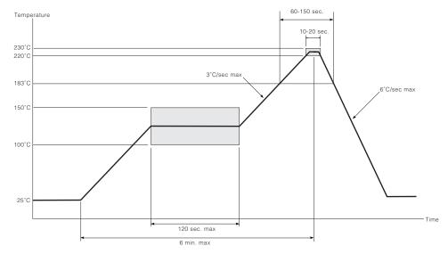
Figure 2-1: Standard Eutectic Solder Reflow Profile (Pb package, Pb paste)
