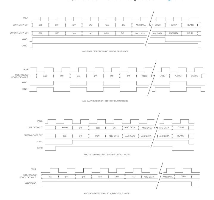
Figure 4-6: YANC and CANC Output Signal Timing
