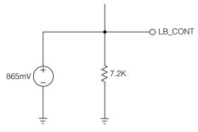
Figure 3-3: PLL Loop Bandwidth Control
