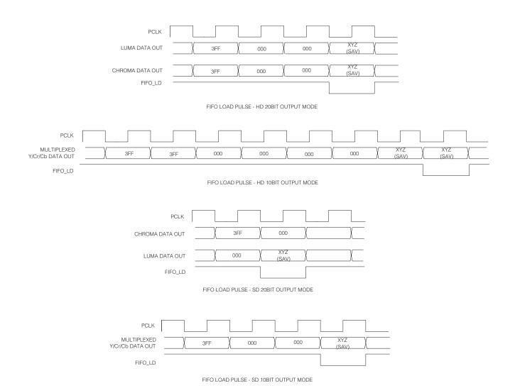
Figure 4-5: FIFO\_LD Pulse Timing
