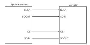
Figure 4-9: Gennum Serial Peripheral Interface (GSPI)
