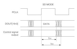
Figure 4-8: SD PCLK to Data Timing
