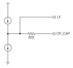
Figure 3-5: VCO Control Output & PLL Lock Time Capacitor
