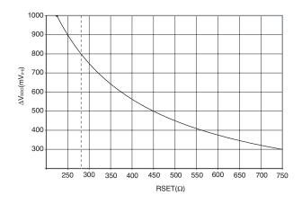
Figure 4-1: Serial Digital Loop-Through Output Swing
