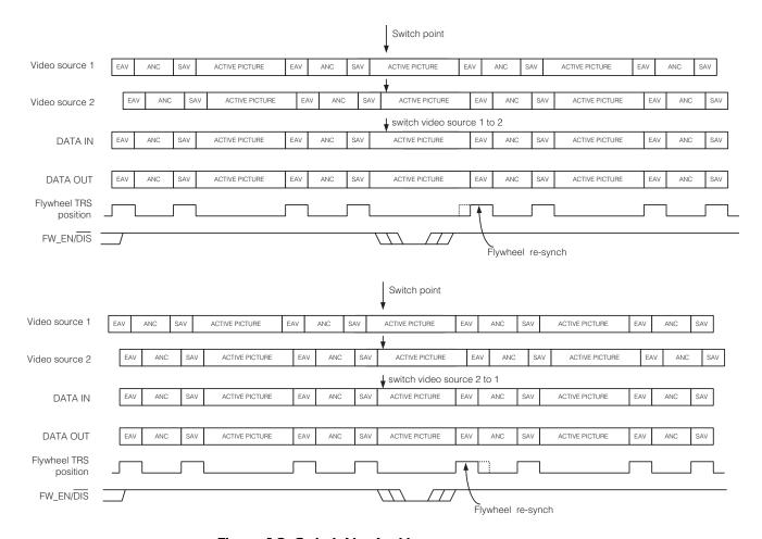
Figure 4-2: Switch Line Locking
