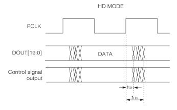
Figure 4-7: HD PCLK to Data Timing
