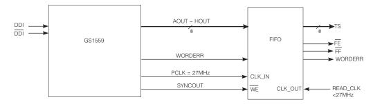
Figure 4-4: DVB-ASI FIFO Implementation Using The GS1559
