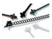
The arrowhead design, in conjunction with the supporting legs or disc, ensure a firm and secure fixing. The disc or legs take up any variation in panel thickness enabling one part to suit many applications. Both the RT and FBS versions are releasable and reusable and the FBS type have the added feature of a ladder type strap as opposed to the conventional serrated strap - this ladder type strap has the benefit of being very flexible.
