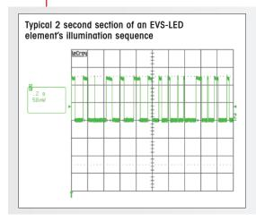
For the EVS system WERMA employs light emitting diodes. A micro-processor generates random light signals. This gives the light a very "agitated" character which proves highly effective in drawing the attention of those in its vicinity — even when seen out of the corner of the eye.
