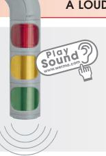
With many applications it is necessary to supplement the optical signal with an additional audible signal. The new LED Beacon and LED Traffic Light from WERMA provide the optimal solution: The high visibility permanent LED light in combination with a loud integrated siren. This combination generates a sound output in excess of 80 dB and a tone frequency of 50 Hz.
