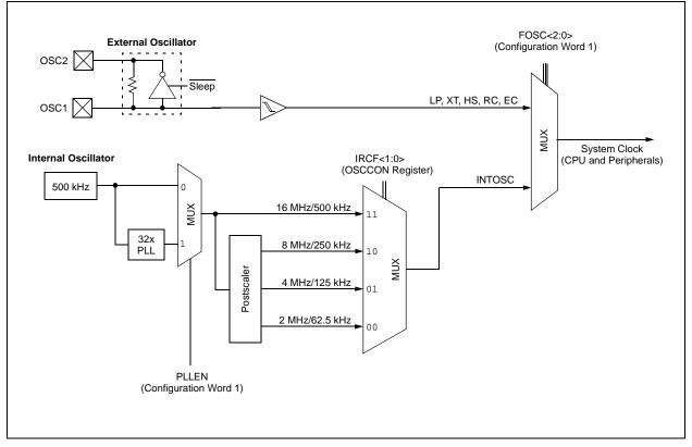
FIGURE 7-1: SIMPLIFIED PIC<sup>®</sup> MCU CLOCK SOURCE BLOCK DIAGRAM
