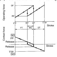
Make sure that the operating body is set so that the actuator should return to the free position when the operating body has moved if a switch is used to form a normally closed (NC) circuit. If a switch is used to form a normally open (NO) circuit, the operating body must move the switch actuator to the distance of 70% to 100% of the rated overtravel (OT) of the switch.
