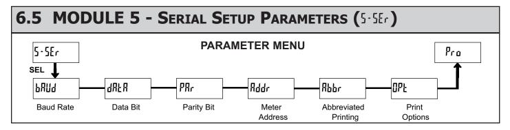
The Serial Setup Parameters are only active when the optional RS232 or RS485 serial communications module is installed in the meter. Refer to the CUB5COM bulletin for complete details on CUB5 serial communications.
