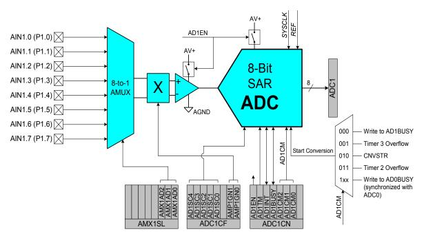
Figure 7.1. ADC1 Functional Block Diagram
