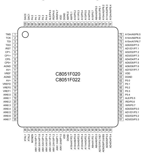
Figure 4.1. TQFP-100 Pinout Diagram
