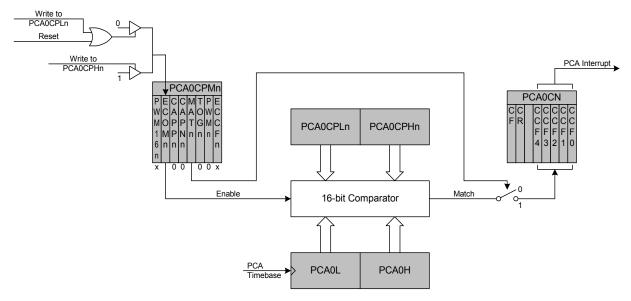
Figure 23.5. PCA Software Timer Mode Diagram
