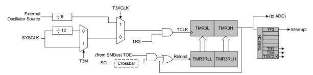
Figure 22.19. Timer 3 Block Diagram
