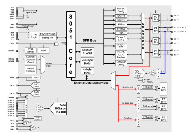
Figure 1.2. C8051F021 Block Diagram
