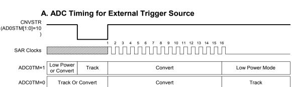
Figure 6.3. 10-Bit ADC Track and Conversion Example Timing
