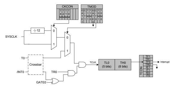
Figure 22.2. T0 Mode 0 Block Diagram
