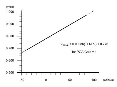
Figure 6.2. Temperature Sensor Transfer Function
