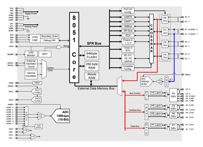
Figure 1.3. C8051F022 Block Diagram
