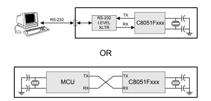
Figure 21.6. UART Modes 1, 2, and 3 Interconnect Diagram
