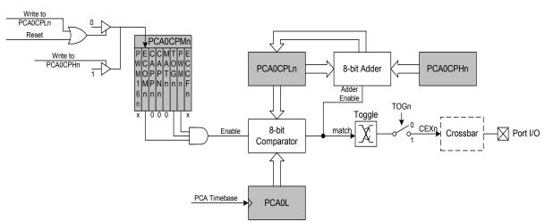
Figure 23.7. PCA Frequency Output Mode
