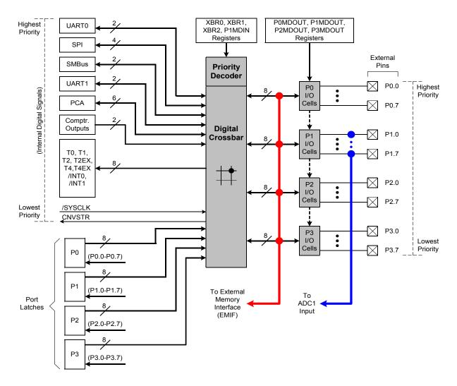
Figure 17.2. Lower Port I/O Functional Block Diagram
