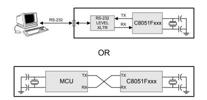
Figure 20.6. UART Modes 1, 2, and 3 Interconnect Diagram
