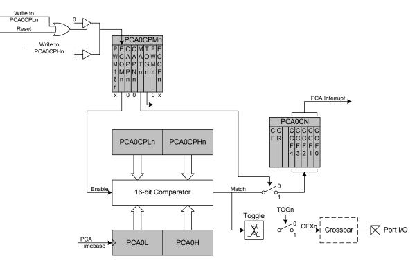
Figure 23.6. PCA High Speed Output Mode Diagram
