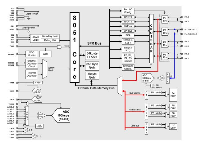
Figure 1.4. C8051F023 Block Diagram
