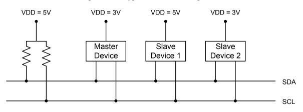
Figure 18.2. Typical SMBus Configuration
