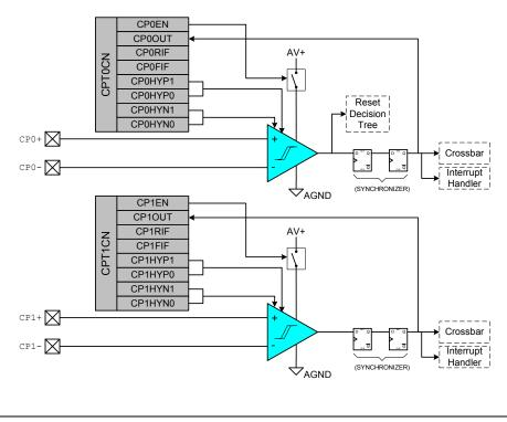
Figure 11.1. Comparator Functional Block Diagram
