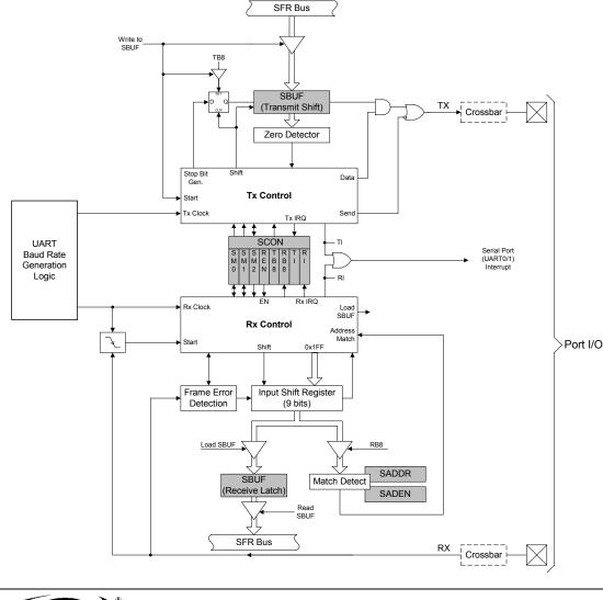
Figure 20.1. UARTO Block Diagram
