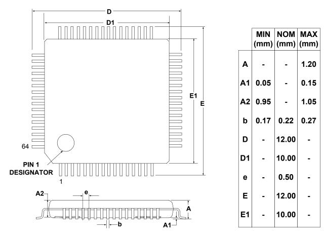
Figure 4.4. TQFP-64 Package Drawing
