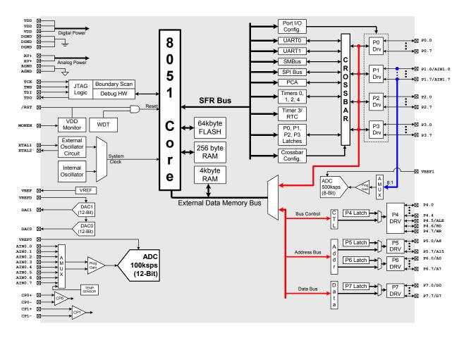
Figure 1.1. C8051F020 Block Diagram
