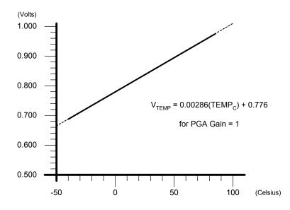
Figure 5.2. Temperature Sensor Transfer Function
