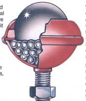
TO DETERMINE BALL UNITS CAPACITY the weight of the article to be conveyed should be divided by 3. The result gives the maximum load which any single ball unit may have to bear. If the Ball Units are levelled accurately, then a larger number than 3 may be applied. The surface hardness and condition of the article to be conveyed should be taken into consideration to avoid undue ball penetration.
