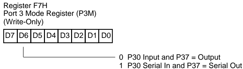
Figure 9-2. Port 3 Mode Register (P3M) and Bit-Rate Generation
