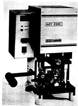
The ACT2500 quickly and reliably crimp terminates up to 1200 contacts per hour. The machine which only requires an electrical supply, is suitable for a wide variety of contacts and cable sizes. Crimp tools are easily changed. Time consuming adjustments are unnecessary, stripping and crimping is sensor released. This semi-automatic crimp machine is a practical and cost saving tool when using Cannon reeled contacts. Please ask for details of our leasing arrangements.
