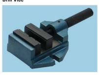
Small drill vice for use in drilling and light milling operations. Effectively grips round, square, thin and irregular sections. The jaws are made of hardened steel and base cast iron. Handle is mounted on ball bearings to give more gripping power, smooth action and long life.
