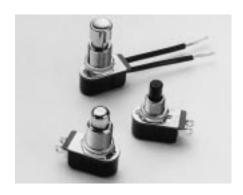
The P26-Series pushbutton switches are single pole, AC rated for 8 amps at 125 VAC and suitable for shallow back panel applications. These switches are momentary action with a medium actuation force (13 oz. typical). The P26-Series switch is equipped with a slowmake, slow-break contact mechanism.
