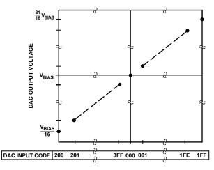
Figure 22. Main DAC Output Voltage vs. DAC Input Codes (HEX) for Twos Complement Coding
