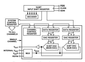
Figure 3. AD7804/AD7808 Internal Registers
