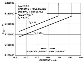
Figure 30. Sink and Source Current at Full Scale with  $V_{\rm DD} = 5~V$
