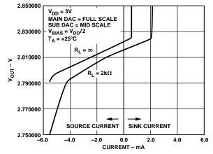
Figure 31. Sink and Source Current at Full Scale with  $V_{DD} = 3 V$
