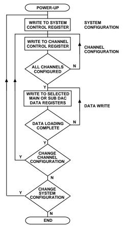
Figure 10. Flowchart for Controlling the DAC Following Power-Up
