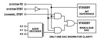
Figure 21. Implementation of Power-Down and Standby Functions
