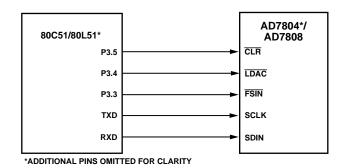
Figure 37. AD7804/AD7808-80C51/80L51 Interface
