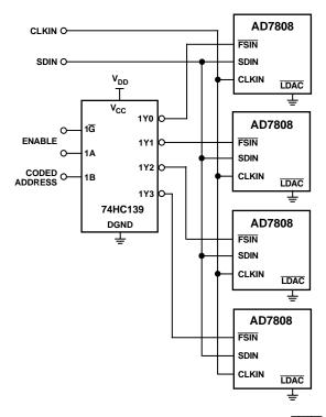
Figure 42. Decoding Multiple AD7808s Using the FSIN Pin
