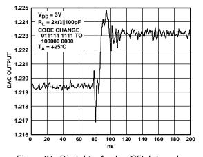
Figure 34. Digital-to-Analog Glitch Impulse
