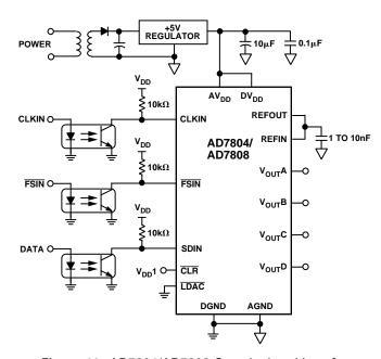
Figure 41. AD7804/AD7808 Opto-Isolated Interface
