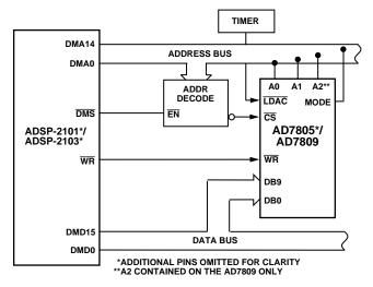
Figure 38. AD7805/AD7809-ADSP-2101/ADSP-2103 Interface
