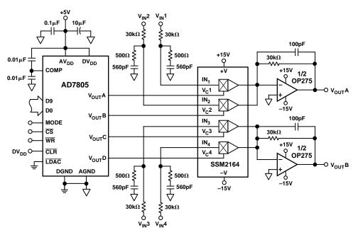
Figure 44. Low Cost, Two-Channel Mixer
