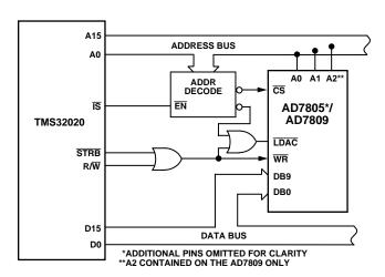
Figure 39. AD7805/AD7809-TMS32020 Interface
