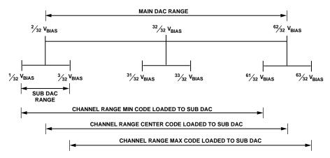
Figure 28. Pictorial View of Transfer Function for Any DAC Channel
