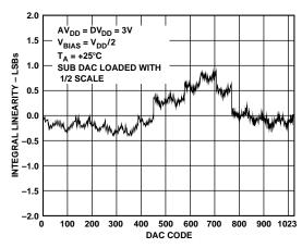
Figure 33. Integral Linearity with 3 V Operation
