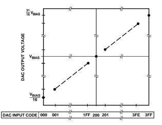
Figure 25. Main DAC Output Voltage vs. DAC Input Codes (HEX) for Offset Binary Coding
