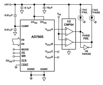
Figure 43. Digitally Programmable Window Detector
