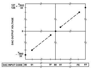
Figure 26. Sub DAC Output Voltage vs. DAC Input Codes (HEX) for Offset Binary Coding
