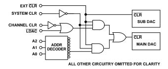
Figure 20. CLR Functions for Main and Sub DACs
