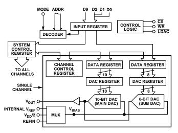
Figure 11. AD7805/AD7809 Internal Registers
