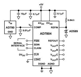
Figure 45. Two Externally Applied References
