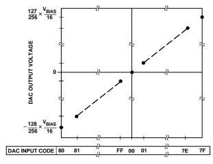
Figure 23. Sub DAC Output Voltage vs. DAC Input Codes (HEX) for Twos Complement Coding
