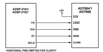
Figure 35. ADSP-2101/ADSP-2103 Interface
