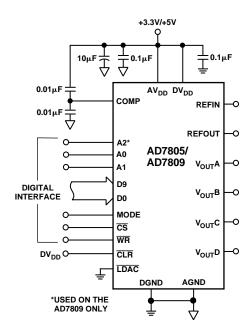
Figure 24. Typical Configuration for AD7805/AD7809
