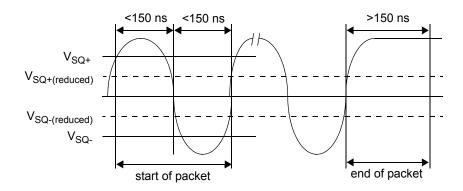
Figure 3-14 10BASE-T Twisted Pair Smart Squelch Operation
