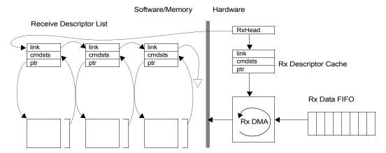
Figure 5-6 Receive Architecture
