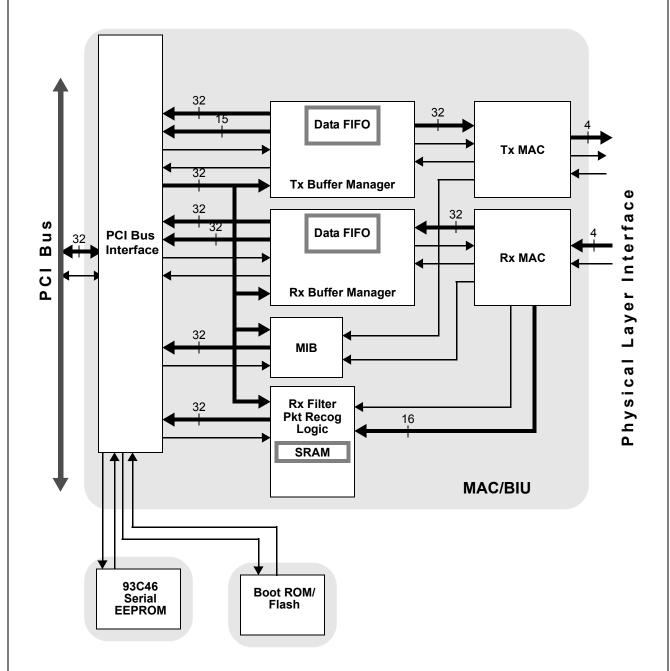
Figure 3-2 MAC/BIU Functional Block Diagram
