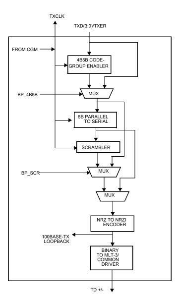
Figure 3-6 100BASE-TX Transmit Block Diagram
