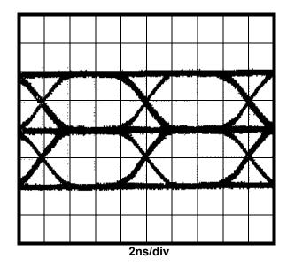
Figure 3-11 MLT-3 Signal Measured at All after 0 meters of CAT  $\underline{V}$  cable
