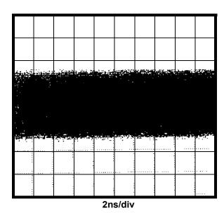
Figure 3-13 MLT-3 Signal Measured at All after 100 meters of CAT <u>V</u> cable
