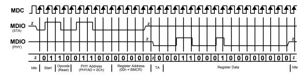
Figure 3-15 Typical MDC/MDIO Read Operation
