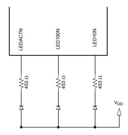
Figure 3-5 LED Loading Example
