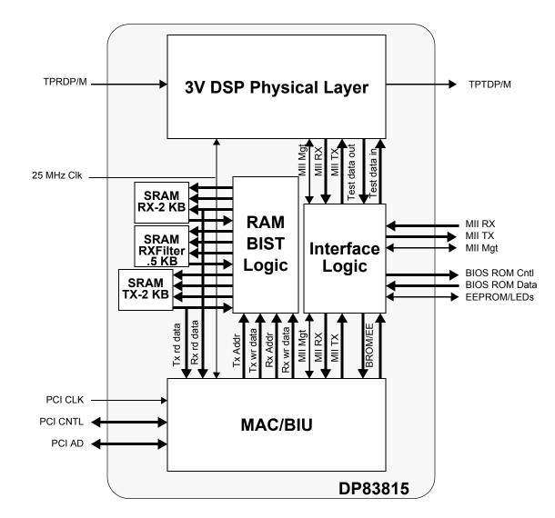
Figure 3-1 DP83815 Functional Block Diagram
