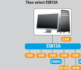
You will obtain the best performance when you do the fewest format conversions. For example, using the E5810A (LAN to GPIB), data transfer will generally be faster than 82357B and an E5813A (LAN to USB to GPIB).
