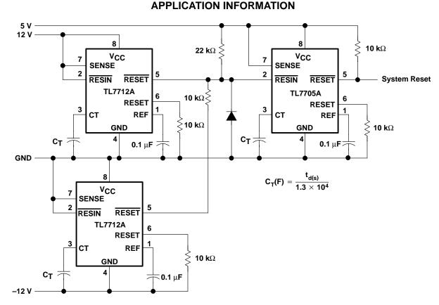
Figure 6. Multiple Power-Supply System Reset Generation
