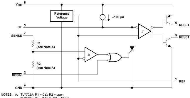
NOTES: A. TL7702A: R1 = 0  $\Omega$ , R2 = open TL7705A: R1 = 7.8 k $\Omega$ , R2 = 10 k $\Omega$ TL7709A: R1 = 19.7 k $\Omega$ , R2 = 10 k $\Omega$ TL7712A: R1 = 32.7 k $\Omega$ , R2 = 10 k $\Omega$ TL7715A: R1 = 43.4 k $\Omega$ , R2 = 10 k $\Omega$
