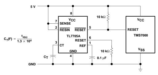
Figure 7. Reset Controller for TMS7000 System
