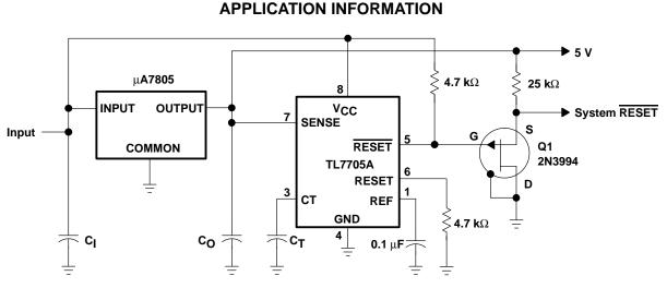
Figure 8. Eliminating Undefined States Using a P-Channel JFET
