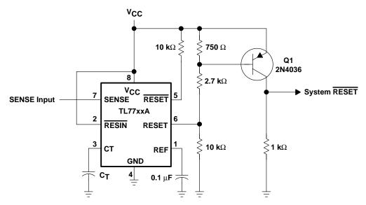
Figure 9. Eliminating Undefined States Using a pnp Transistor
