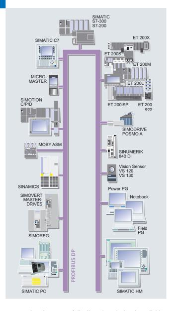
A comprehensive range of distributed I/O devices is available. SIMATIC ET 200 can offer the right device for any application:
