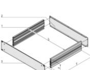
$\begin{array}{l} h = clearance \; (height) = H\text{-}8,1 \; mm, \; b \\ = clearance \; (width) = 403 \; mm \end{array}$
