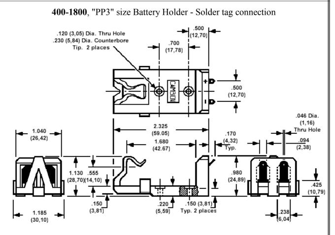
Rec. Mounting Holes - .062 (1,57) Dia., on pitch of 0.500 (12,70) centres, plus bolt down holes per drawing Suited for use on boards up to .125 (3,18) thick
