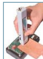
Verify the effectiveness of shielding
