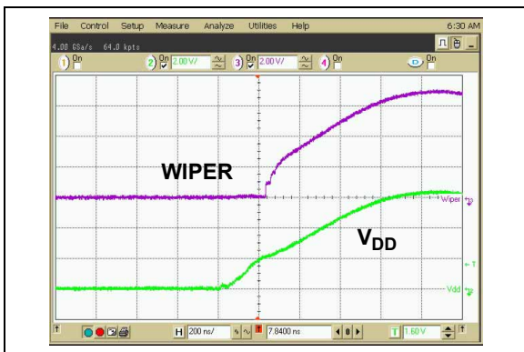
FIGURE 2-15: 2.1 k \Omega – Power-Up Wiper Response Time.
