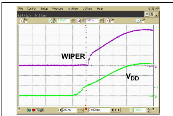
FIGURE 2-52: 50 k \Omega – Power-Up Wiper Response Time.
