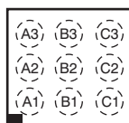
YFF PACKAGE 9-BALL WCSP (TOP VIEW)
