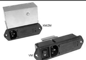
**FM Models** – General purpose RFI filter designed for susceptibility applications, effectively providing RFI control of line-to-ground noise. The design is compact and meets the very low leakage current requirements of VDE portable equipment as well as (120 Volt) UL544 non-patient medical equipment.
