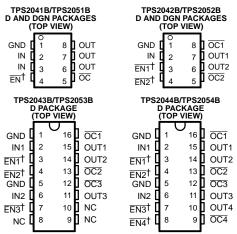
$^\dagger$  All enable inputs are active high for the TPS205xB series. NC – No connect
