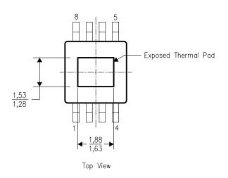
NOTE: All linear dimensions are in millimeters
