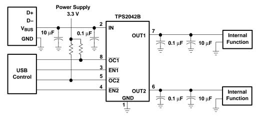
Figure 32. High-Power Bus-Powered Function (Example, TPS2042B)
