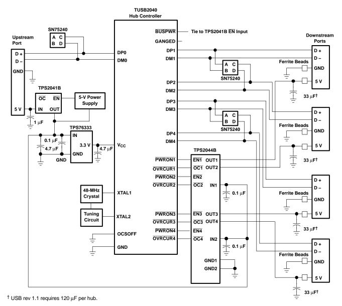
Figure 36. Hybrid Self / Bus-Powered Hub Implementation, TPS2044B/TPS2054B
