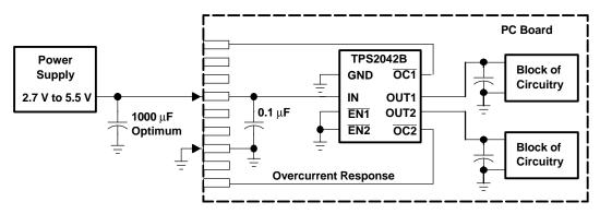
Figure 37. Typical Hot-Plug Implementation (Example, TPS2042B)
