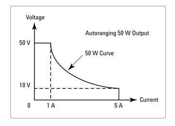
Therefore, this 50 W autoranging power supply, due to its extended voltage and current range, can produce voltage and current combinations in the range of a 250 W non-autoranging power supply.
