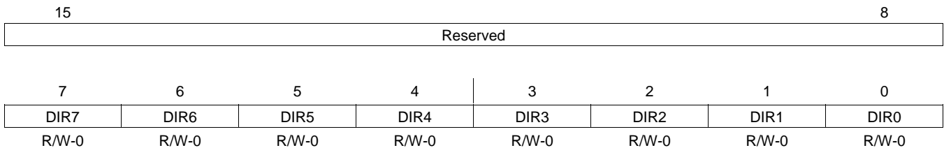
Figure 3-23. General-Purpose I/O Control Register (GPIOCR) [MMR Address 003Ch]
